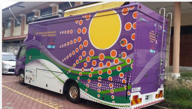
CETREE GREEN TECHNOLOGY LORRY (VEGETABLE OIL BASED GENSET – 8 Kwh)- Biodiesel
